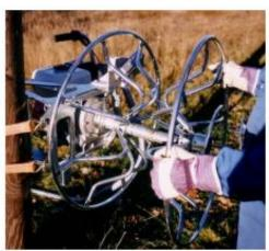
After lifting out the coil of old conductor, re-install the drum gable. Now the drum is ready for re-use.
