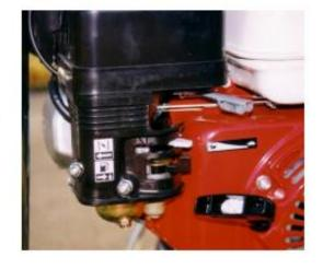
CAUTION: Never pull out the starting cord fully, or allow the starting handle to snap back. Retrurn it gently to its original position.
