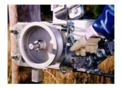
Fold up the locking arm and secure it with the eccentric locking device. Make sure that the pipes lie correctly with the milled opening in the gearbox. Fit the capstan wheel onto the output shaft from the gear. Secure with the locking pin
