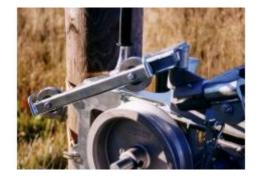
Install the line spreader on the attachment for the input roller. Always use the line spreader for line pulling.
