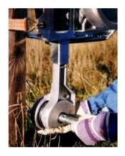
Install the drum holder on the engine bracket slide it up to its highest level to simplify installation of the drive belt.
