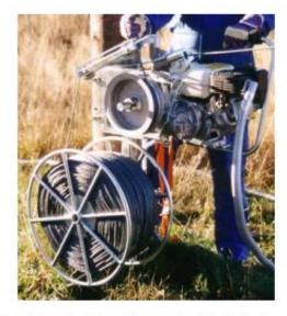
A line drum is used for all kinds of line and suspended cable pulling. The drum should only be used with original 3-ply Polynite with a minimum ultimate breaking load of 800 kp. (6 mm, length 550 m or 1100 m). Please contact SAHLINS SWEDEN AB if any other kind of line is used. Use swivels between the pilot rope and the conductor. Lines must only be spliced by using approved splices.
