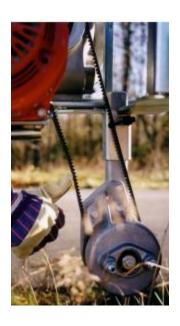
Put the drive belt over the drive pulley on the gear, and the pulley on the drum holder.
