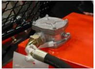
Always pour in new oil through the filter, up to the top level mark on the tank.
