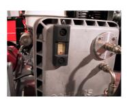
set on the dynamometer. Remove the centre cap and the red indicator is then turned using the attached key. Press down while turning (9).
