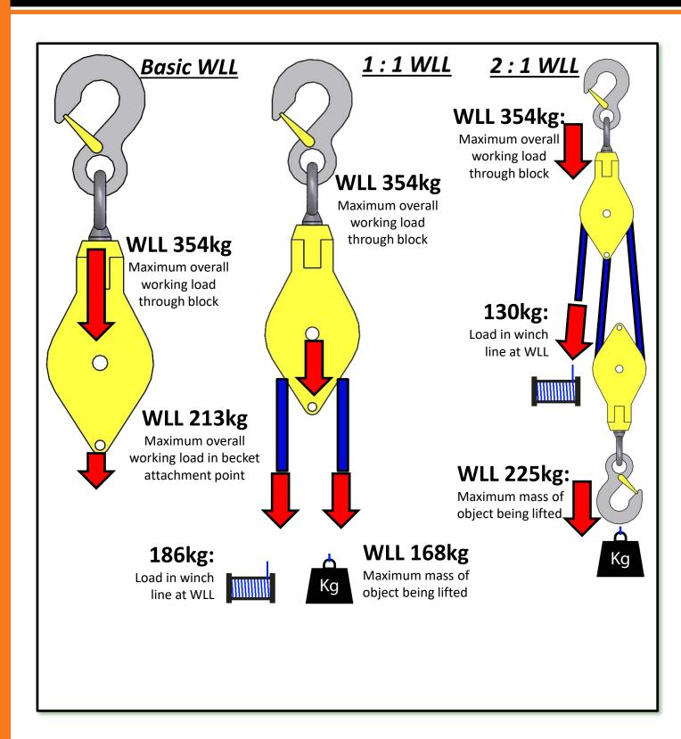
Note: All calculations assume approx. 10% frictional loss around each sheave when used at the WLL
