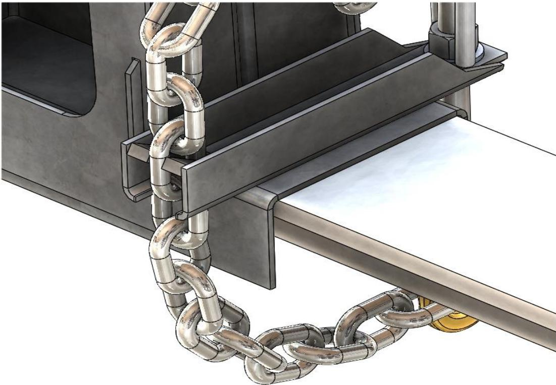
Hook both hooks on spreader bar under the conductor and slowly raise by reversing direction of winch handle rotation. Only raise until hooks seat under conductor.
