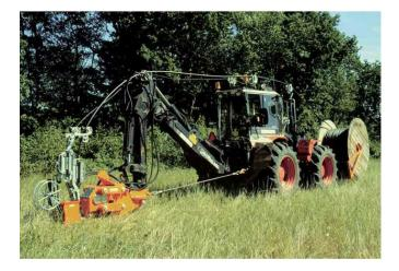
Vibrating ploughs can cope with difficult soil conditions and are more lenient on the cable. Stones and small rocks are disposed of more easily and the furrow is filled again with fine grain material.
