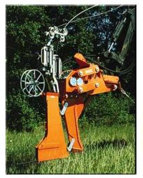
The plough can be equipped with Sahlins hydraulic feeders and slitsing system. With this unique method the fibre optic cable is laid in a protective polyethylene pipe in one operation as it being ploughed into the ground. The polyethylene pipe is being slitted in the slitting unit and the cable is automatically put into the pipe. Thanks to the built in tension in the polyethylene pipe it always closes the slit before it goes down through the chute.
