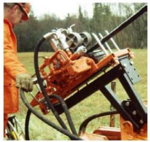
Hydraulically operated feeding unit for power cables. Three cables can be fed simultaneously.
