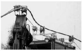
Cable rollers for roof of tractor and backhoe/loader arm. The rollers are available in a suitable version to match the tractor and cable in question.
