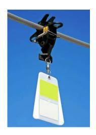
The "FireFly"™ BFD has a salt spray and weather resistant stainless steel ball bearing swivel allowing the diverter to spin in wind speeds as low as 3-5mph. This spinning action combined with the 3-in-1 fluorescent colours reflecting UV and visible light, specific to avian vision, increases the diverter visibility by creating a flashing effect as seen by the bird up to a quarter of a mile away alerting it to the obstruction.
