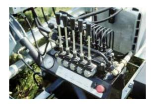
All controls are concentrated on the left side of the machine. Indicator (dynamometer) for pulling force is located under the hydraulic controls.
