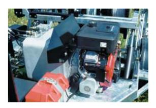
The power comes from petrol driven hydraulic power pack, with built in cooling fan to guarantee safe and long time working.
