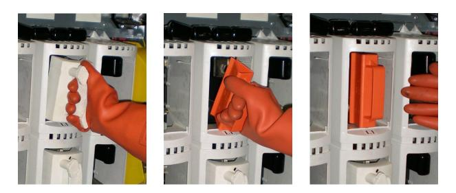
As the unit is moulded as a single piece from Orange FR Polymer ABS Plastic, they have a robust handle for safe fitting and removal. Length is 138mm. The covers can be supplied with individual 1000V dielectric testing.
