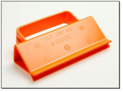
These fuse shields are designed to fit over fuse contacts when the fuse is removed in locations such as take off chambers, open boards, LV pillars and path boxes providing protection against accidental contact with the fuse contacts up to 1000V. The cover also provides a safe protection against a phase to phase or phase to earth situation when a temporary or permanent LV open point is in place.
