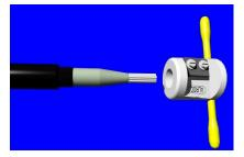
Once insulation has been exposed, fit the TC tool on the end of the cable and rotate handles to create a clean taper on the insulation.
