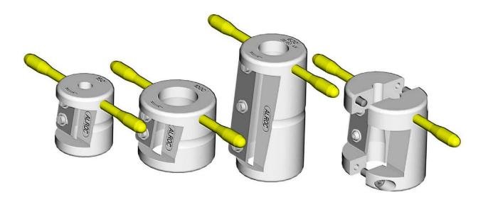
The TC range of Alroc tools enable an exact length of insulation to be tapered on MV cables. Simple to use operating in a similar fashion to a pencil sharpener, the tools are non adjustable and are manufactured to suit individual cable specifications.
