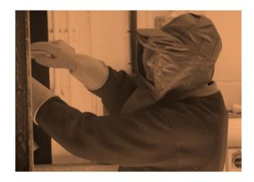
The Clydesdale Arc Flash Hood with Ear Protection is designed to protect the wearer's head and neck from the thermal effects of an electric arc flash, should one occur whilst working under live conditions, such as fault-finding.
