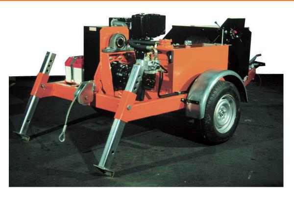
The underground cable winch 3300 is a hydraulically operated 3 tonne winch with a variable pulling speed and force.
