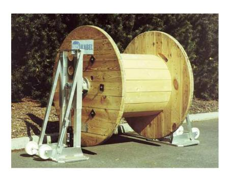
Clydesdale aluminium lightweight drumstands are ideal for use in yards and depots. Fitted with wheels for easy manoeuvring, they have large baseplates making them very stable and easy to set up. The shaft is fitted with slide bearings for easy rotation and locking collars double as centring devices to ensure the shaft is in the centre of the drum to improve stability under pay-out. The robust hydraulic jacks have chrome plated pistons for corrosion resistance
