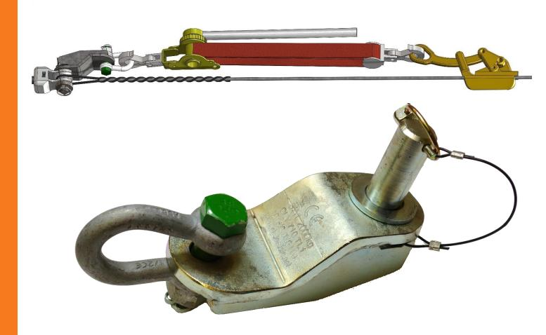
The TL1 Linkage is designed to assist in the tensioning of overhead lines before applying helical ties. It allows the puller and associated tensioning gear to be offset to one side of the conductor and insulator allowing better access for applying preformed terminations.
