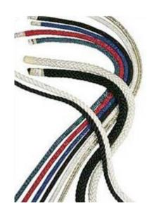
Paracore has a relative density of 1.38 and can be used in extremes of temperature from -70 deg C to +200 deg C, however, extremely high temperatures (over 100 deg C) will reduce MBL. Paracore is supplied as standard with soft eyes at each end unless requested otherwise.
