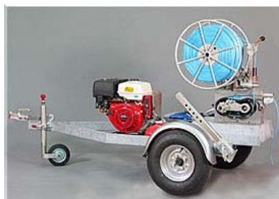
The drum here is a split drum for dismantling old line.
