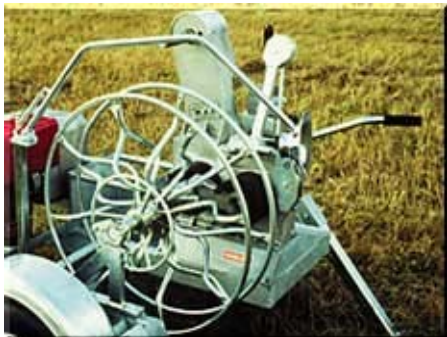
The drum here is a split drum for dismantling old line.
